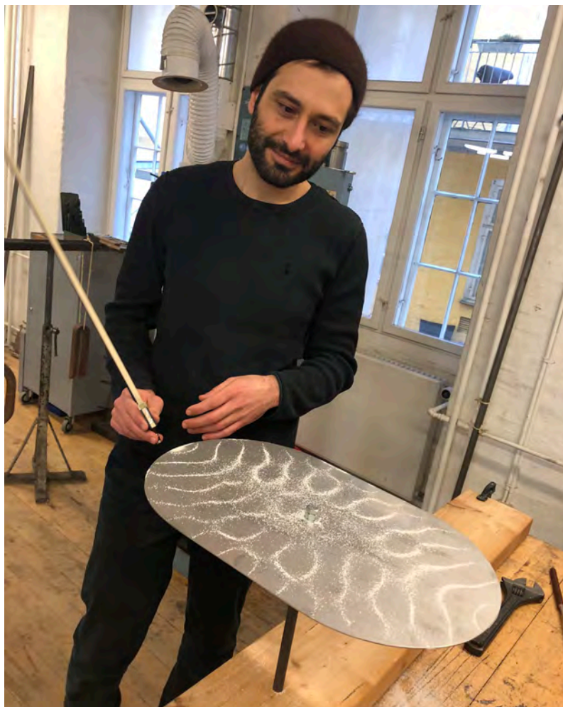
Building and testing the Chladni Plate, a device that reveals vibrational patterns of sound
